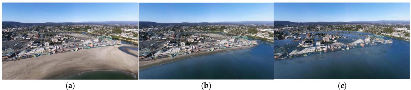
Figure 6. Cropped views from the 360° aerial images of Main Beach, Santa Cruz, CA included in the SLR Explorer Santa Cruz; (a) summer of 2019; (b) king tides, 2019; (c) 0.73 m of SLR combined with 100-year storm.
